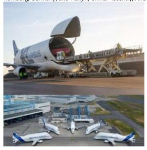
The Beluga XL can carry two A350 wings in one load. Photo: Airbus
