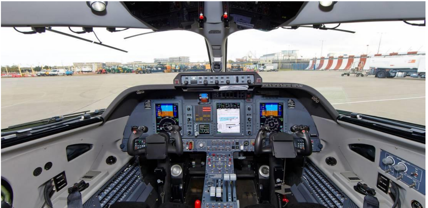
The front office of the Avanti Evo is the Rockwell Collins Pro Line 21.
