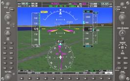
**Under-speed Protection** (USP) is an intuitive flight director function that reacts to under-speed conditions in a way that allows the autopilot to remain engaged, but prevents the airplane from stalling.
