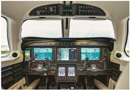
G3000 in the M600 features three main flight displays with split presentations that allow for seemingly endless configurations of information and data. For example, the PFD can be split 60-40 to show the primary view, with speed and altitude tapes next to the digitized Jeppesen approach plate.
