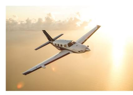
Redesigning a clean-sheet wing lead to performance improvements and the M600's new wing carries an impressive 90 gallons more Jet-A compared to the original.
