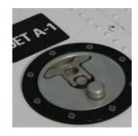
Piper Aircraft launched early 2014 a diesel version of the Archer at the Aero Friedrichshafen in Germany which is powered by a Continental / Centurion 2.0S JET-A compression-ignition engine. Since receiving it's EASA STC in Europe several aircraft have been delivered to various flight schools in Europe.
