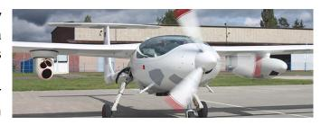
Mission capabilities of an endurance of up to 20 hrs, payload up to 770 lbs and a range of up to 1,350 nm at near stealth quality are impressive values of this aircraft.
