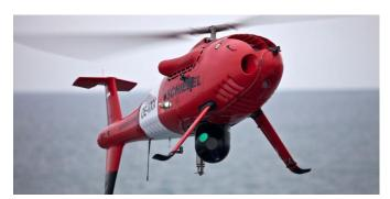
During a flight demonstration held at De Kooy Airfield in Den Helder, the Netherlands, in December, Schiebel supplied an S-100 fitted with the NLR-developed AirScout detect-and-avoid system. A Coastguard Dornier Do-228 fixed-wing turboprop and an RNAF Alouette helicopter acted as "intruder" aircraft for the system to detect. The air force also provided ATC services.
