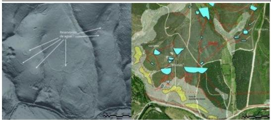
These are ancient goldmines in the Eria river valley, with channels and reservoirs for exploitation. The model generated with LiDAR data (left) allows these structures to be located on aerial photos (right).
