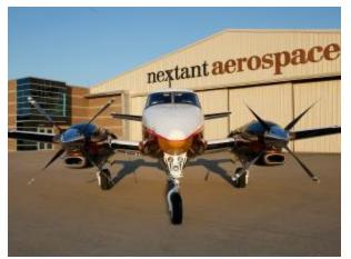
Nextant Aerospace has received FAA certification for the **G90XT**, a remanufactured Beechcraft twin turboprop with GE H75 engines, an avionics suite based on Garmin's G1000 and new paint and interior.
