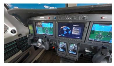
single-engine turboprop to feature Garmin G3000 in the cockpit, the M600 is equipped with the most sophisticated avionics and safety features available. A touchscreen-controlled, all-glass flight deck offers the most comprehensive and technologically advanced package, listed at a competitive price for 2016 of \$2.85 million.
