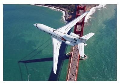
The Falcon 8X represents something of a paradigm shift for Dassault. This is the first time in the company's history that it has stretched one of its existing Falcon Jets to create a derivative model rather than embark on a clean-sheet design. Two 21-in. barrel plugs, one ahead and one aft of the wing root, were added to the 7X fuselage. The modification makes room for two additional windows on each side of the fuselage and adds about 3.5 ft. to cabin length. The stretch also makes room for a
