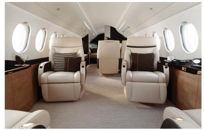
Forward section of the cabin has four-seat club grouping with 20-in. wide chairs. A new acoustical insulation package is expected to lower cabin sound levels by 2 to 3 db while reducing completion weight by up to 500 lb. Credit: Dassault Falcon Jet
