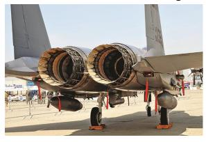
GKN Aerospace Chem-tronics has been selected by Tinker Air Force Base, Oklahoma, to supply 147 turbine nozzle support structures for the Pratt & Whitney F-100 series engines that power <u>USAF F-15</u> and <u>F-16</u> aircraft. This contract is valued at approaching US\$10 million. These titanium alloy structures support the aft nozzle exit section in the rear of all F-100 powerplants. Manufacturing will take place at the company's El Cajon, California, facility, with
