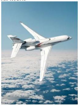
Eric Gérard's aerial ballet in the Falcon 8X, particularly slow speed maneuvering, is impressive to watch from the ground, giving potential corporate pilots the confidence to take off from runways as short as 6,000 ft. and, when necessary, land on runways as short as 2,150 ft. with eight passengers and NBAA IFR reserves.
